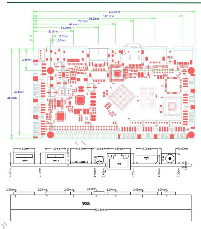
PCB size: 126.5mm\*70mm/±0.5mm; board thickness 1.6mm±10%
